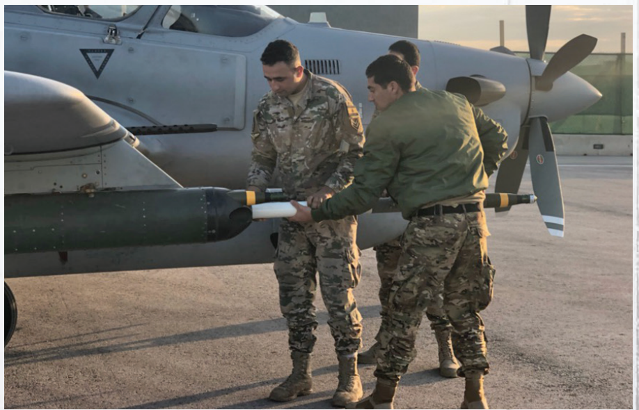
Lebanese Air Force armament crews load AGR-20s on an Embraer A-29 Super Tucano. CAA aircrew and JTACs worked closely with LAF aviators learning to employ the laser-guided rockets. (Photo courtesy of Lt Col Brian Raridon)
